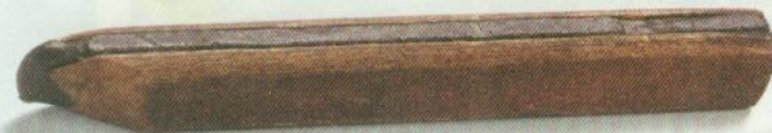
The oldest known pencil (found in a timber-frame house built in 1630) reveals its graphite-sandwich construction. The shape resembles today's carpenter-pencil design, which woodworkers and carpenters appreciate because the flat sides prevent it from rolling off of roofs and workbenches.
